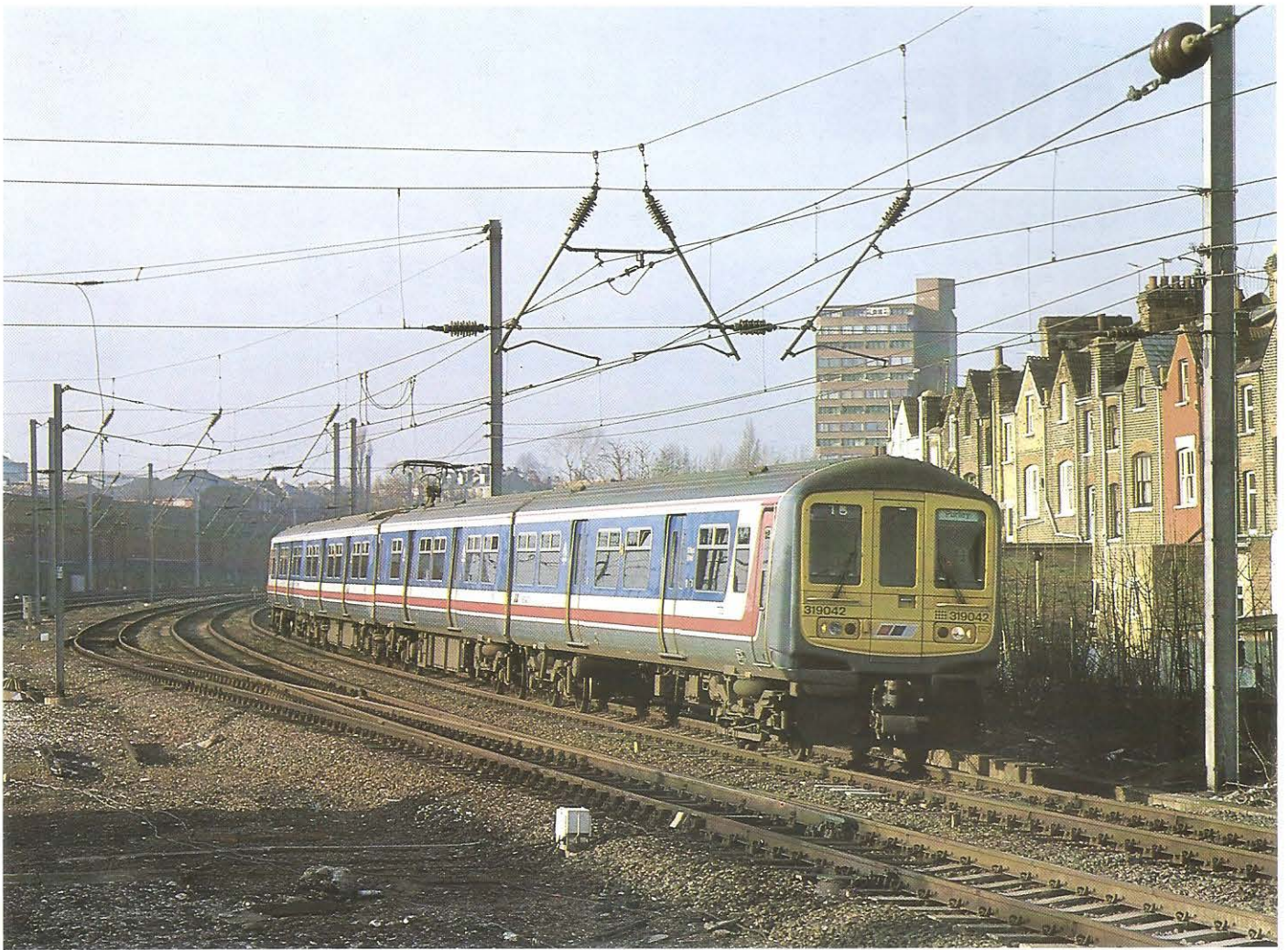
A Thameslink train operating from the 25kV supply in the north London suburbs.
